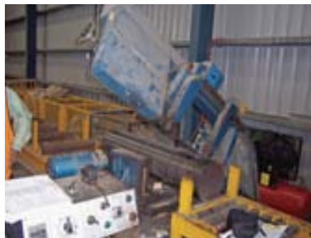
The band saw and line pipe that was being cut at the time of the accident
