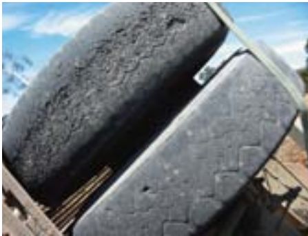
Close up of the left rear inner and outer tyres of the trailer, with the wire belting showing on the outer tyre
