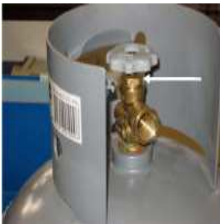
Valve showing loose gland nut
